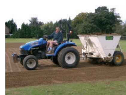
3. Spreading and integrating cricket loam
